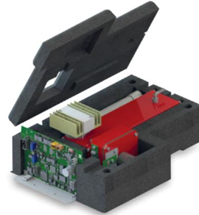
Great accuracy: the measuring module and correlation wheel are set in the enclosed foam box for stable temperature and no interference from external conditions
