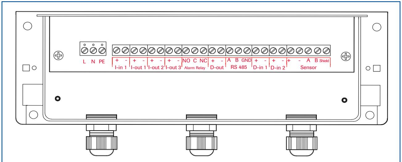
Fig. 13: Electrical connection for MSE 300 in the field housing
