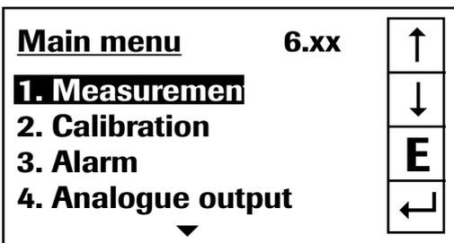
To access the main menu, press and hold any area of the display for several seconds. The sub-menu selection appears.
