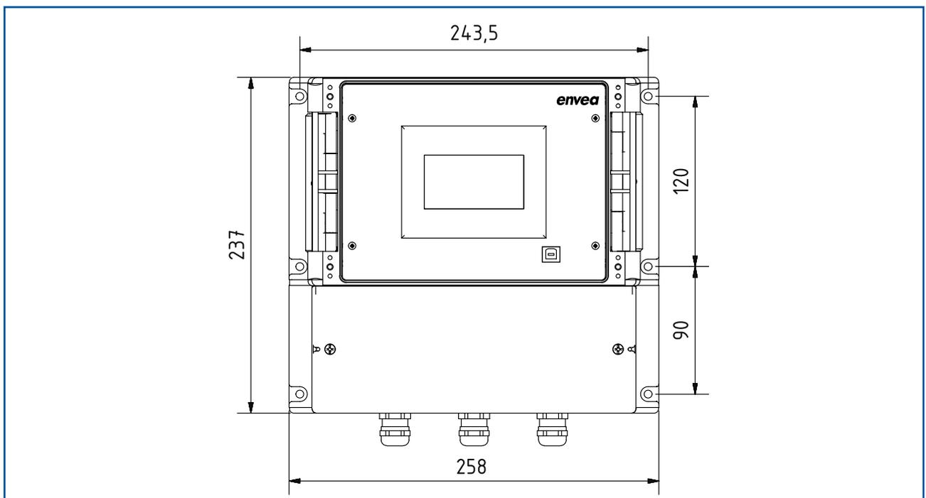
Fig. 6: Dimensions of the MSE 300 in the field housing (front view)
