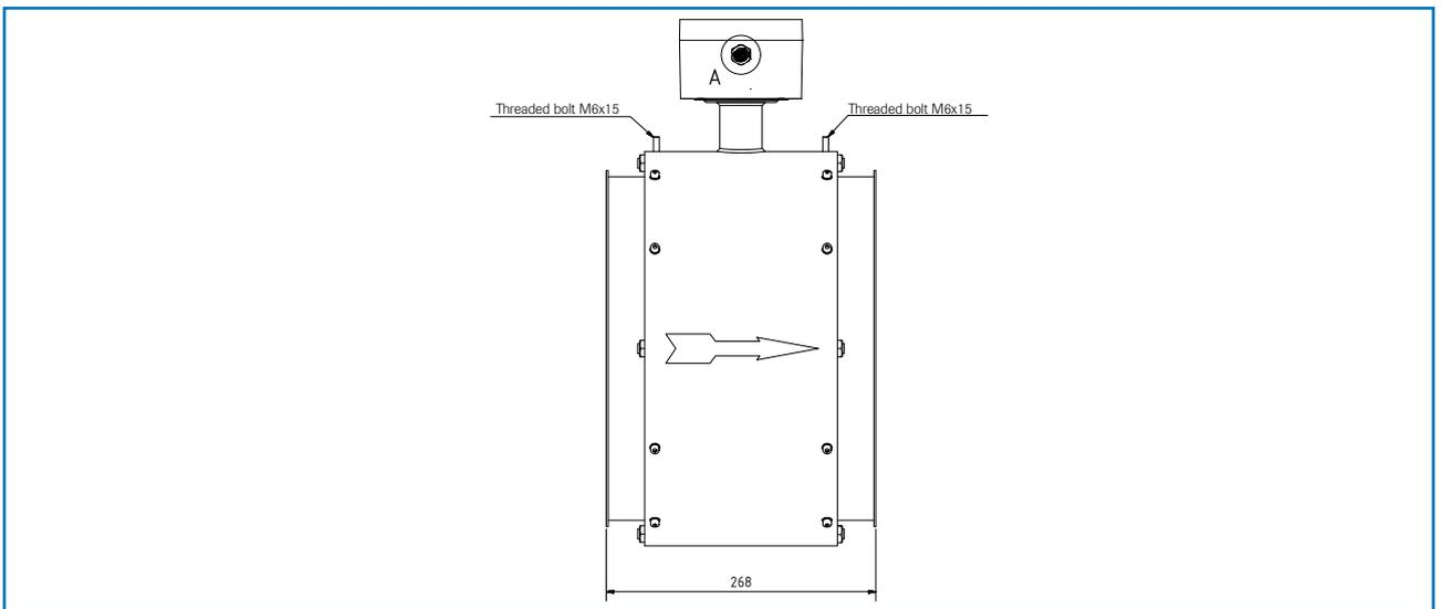
Fig. 9: Dimensions of the SpeedFlow 2.0-Pipe sensor
