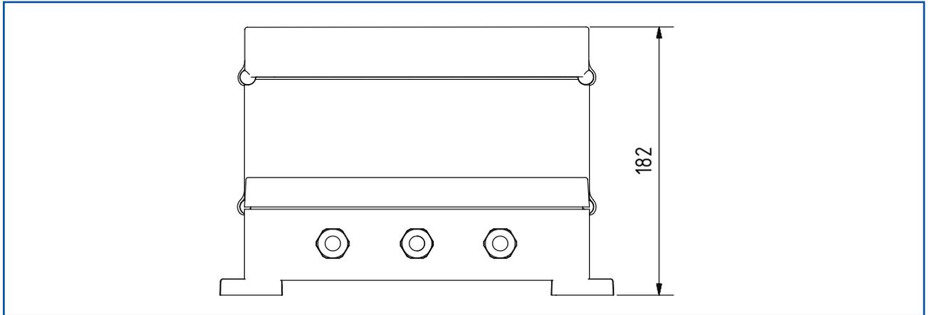
Fig. 7: Dimensions of the MSE 300 in the field housing (side view)
