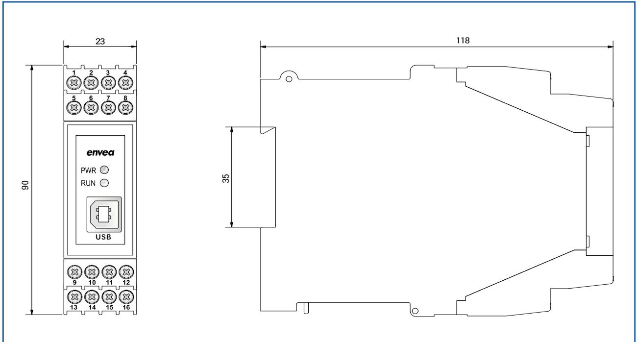
Fig. 5: Dimensions of the MSE 300 in the DIN Rail housing
