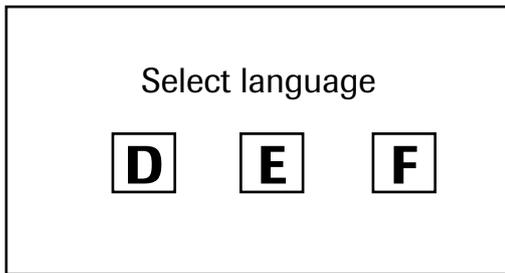
Initialisation screen the first time the MSE 300 in the field housing is switched on.
