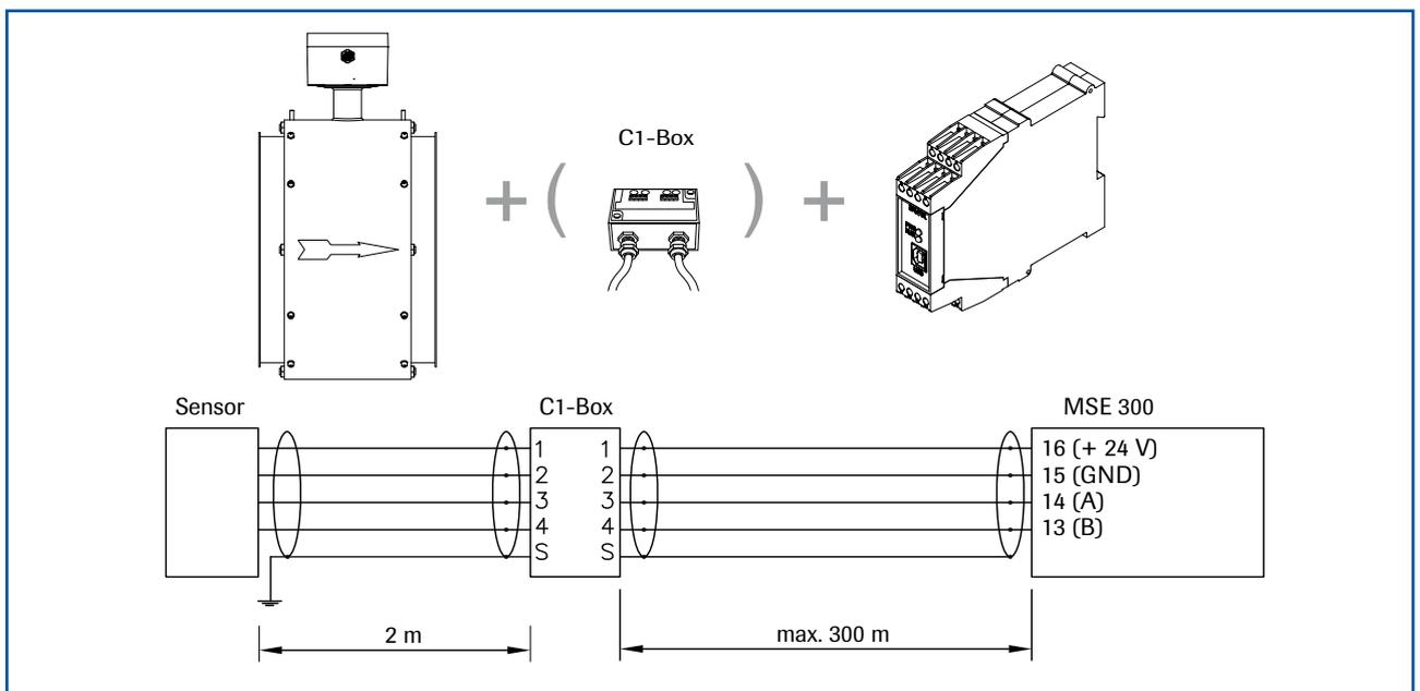
Fig. 2: Overview with C1-Box and DIN Rail
