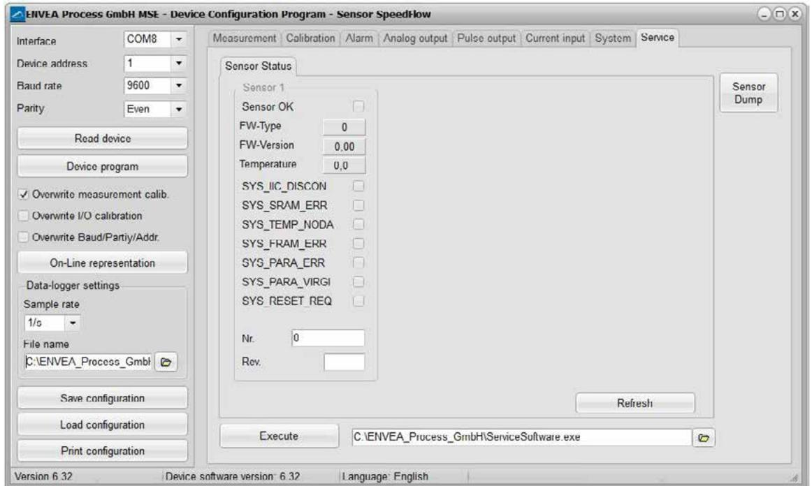
In menu **8. Service** the status of each connected sensor is displayed. FW type, FW version, temperature, serial number and possible hardware errors are automatically read in and displayed. In the case of a change of display, the PC software can be used to adjust the contrast, if necessary.
