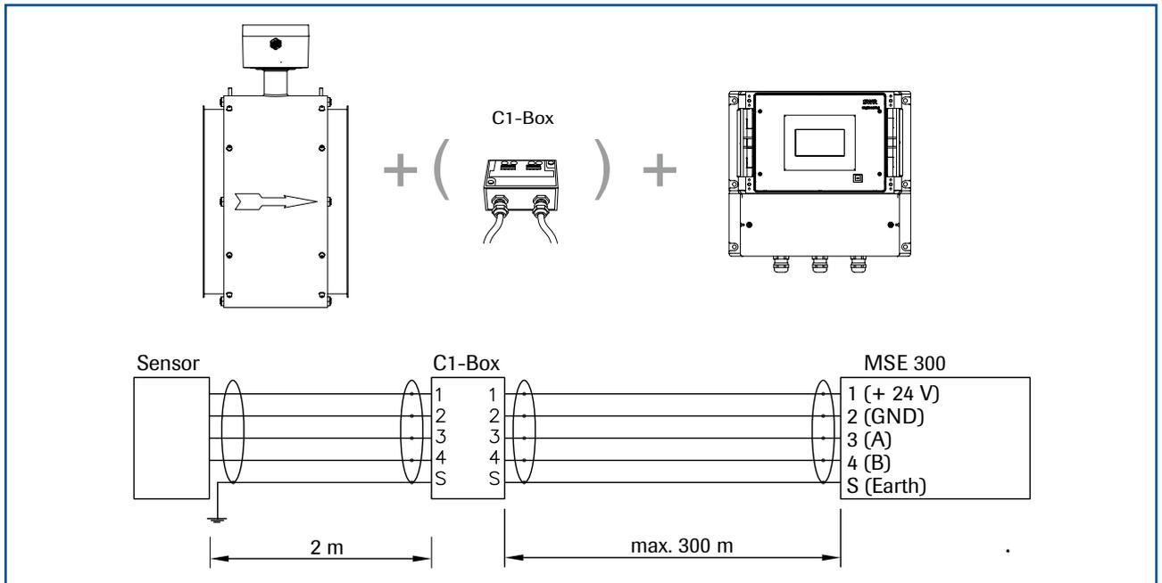
Fig. 1: Overview with C1-Box and field housing
