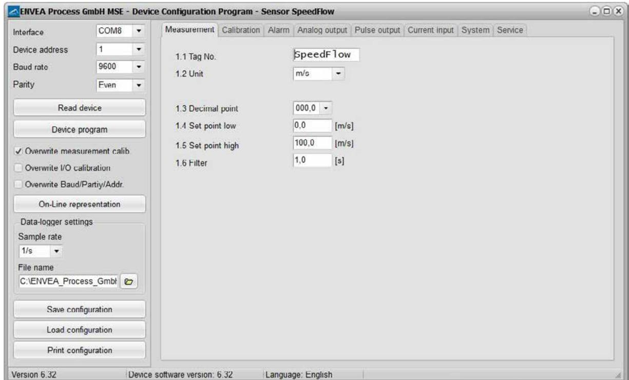
Communication is established by clicking on “Read device”. The acknowledgement message “Parameter read in” is displayed. If an error message is displayed instead, check the communication parameters and cable connections between the PC and the Evaluation unit.
