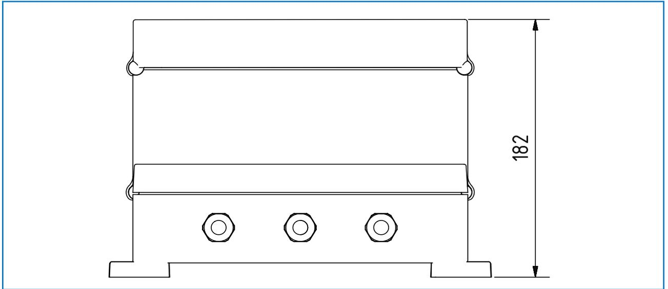
Fig. 9: Dimensions of the MSE 300 in the field housing (side view)
