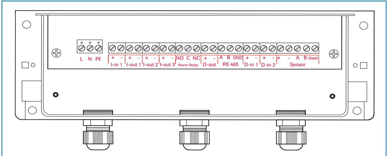
Fig. 13: Electrical connection of MSE 300-FH
