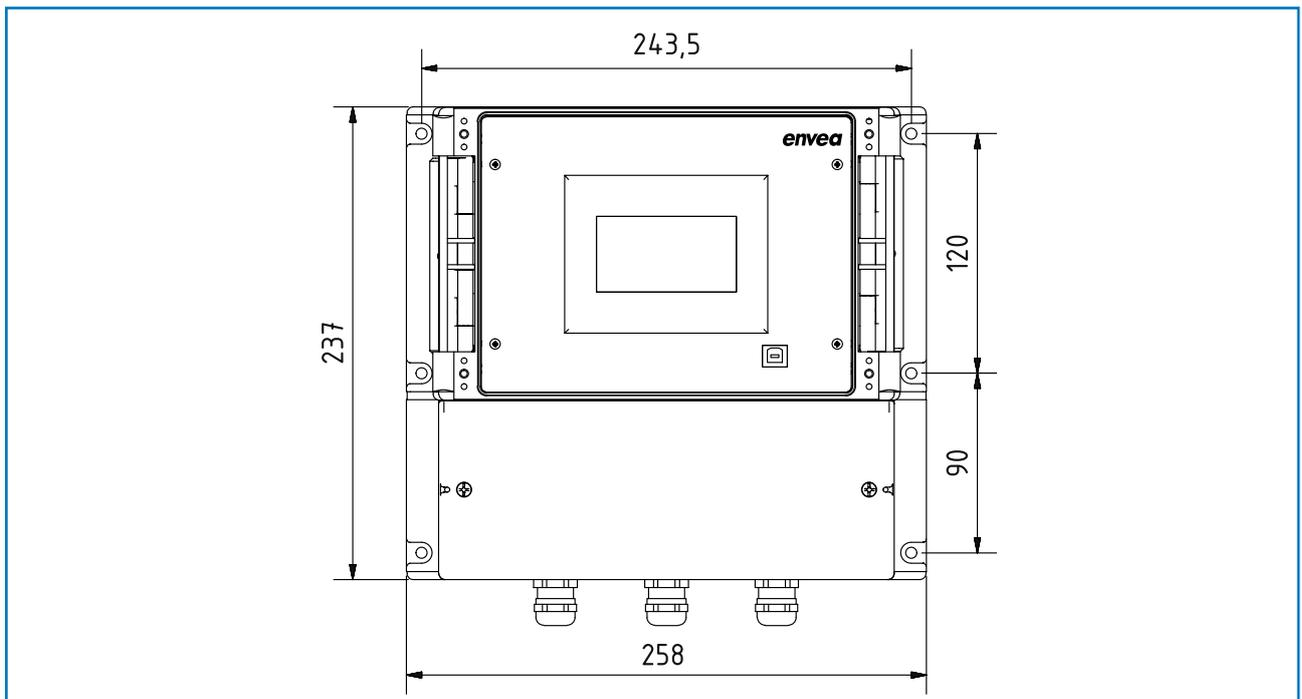
Fig. 8: Dimensions of the MSE 300 in the field housing (front view)
