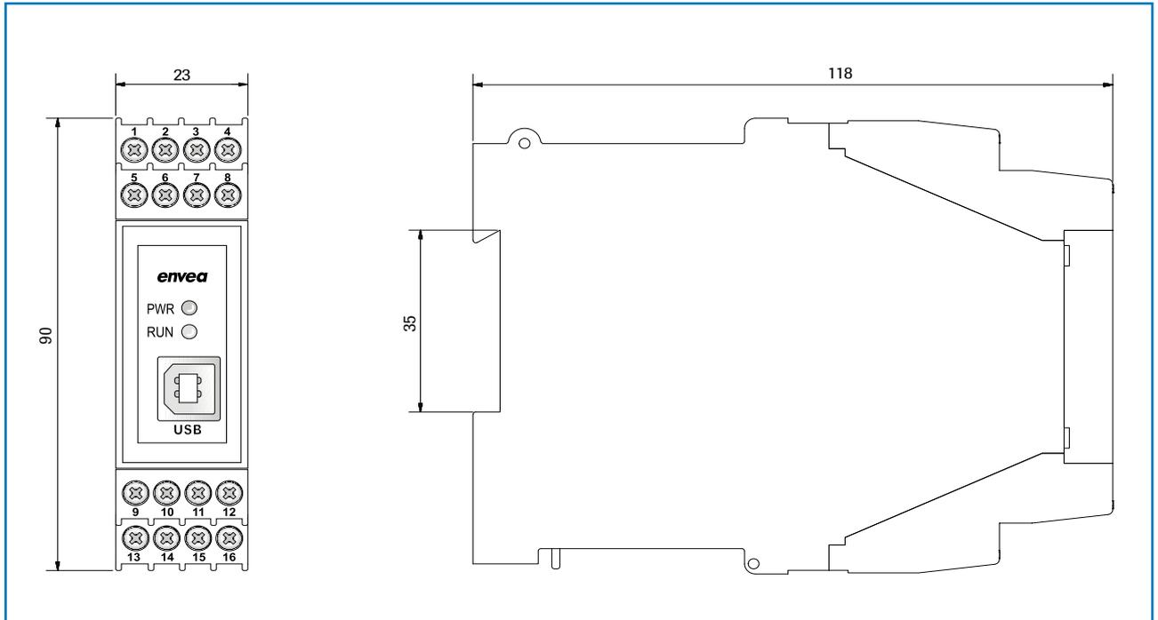
Fig. 7: Dimensions of the MSE 300 in the DIN Rail housing
