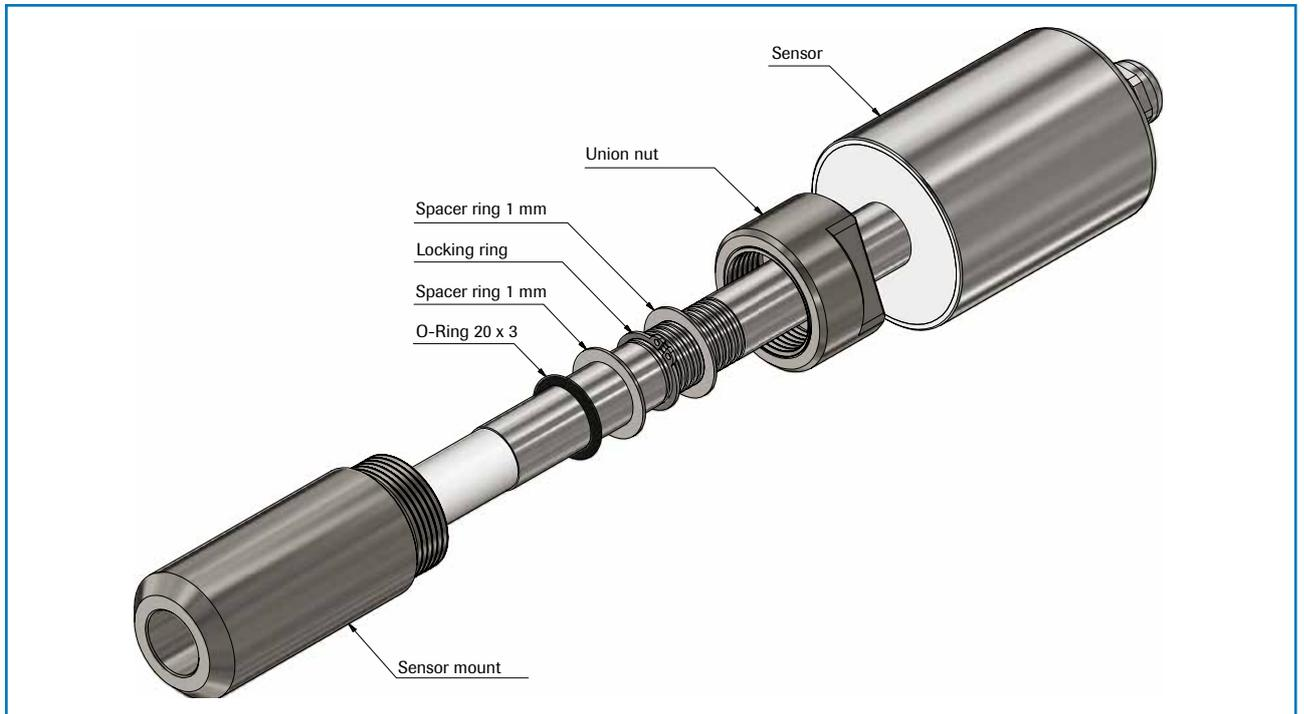
Fig. 6a: Installation of sensor in the sensor mounting
