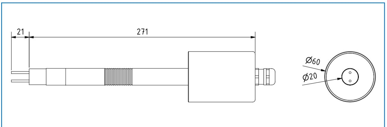
Fig. 11: Dimensions of the SpeedFlow 2.0 sensor
