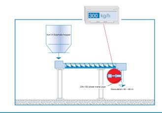
An analogue output with 4 ... 20 mA, a changeover relay contact as well as a pulse output (open collector) are available for the evaluation of the sensor signals.
