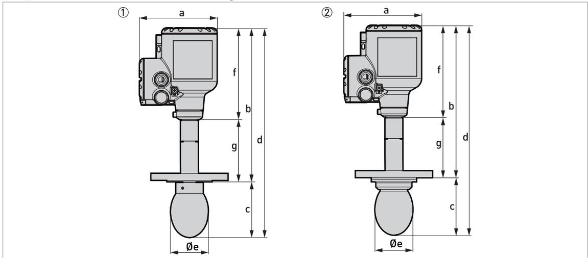
Figure 8-14: Drop antennas with standard flange connections
