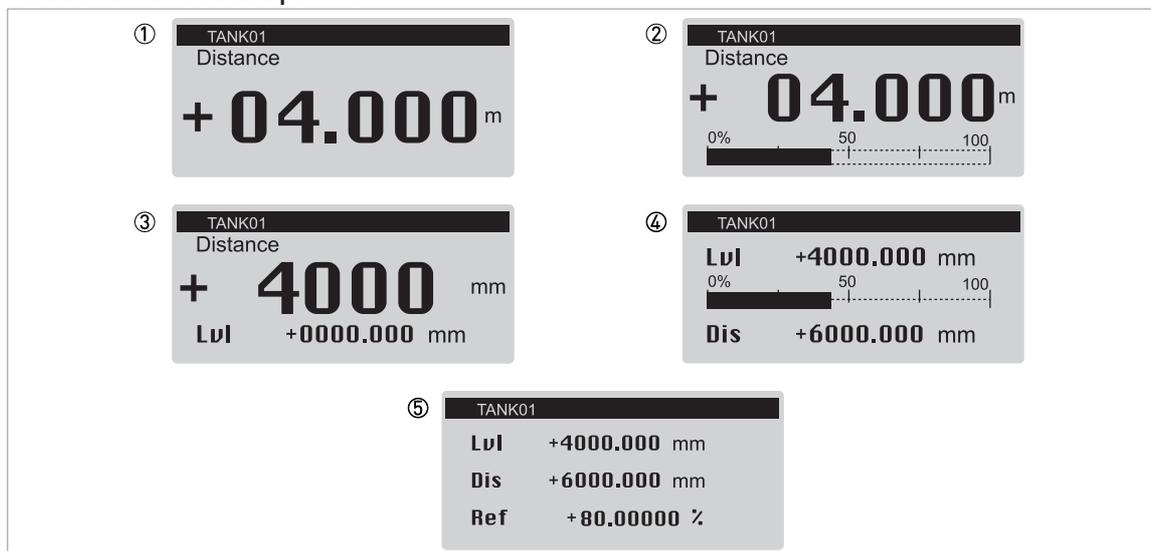
Figure 6-1: Measurement data options in Normal mode
