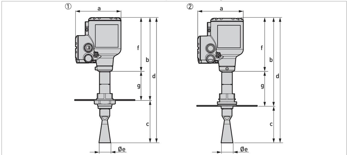
Figure 8-12: Metallic Horn antennas with low-pressure flange connections
