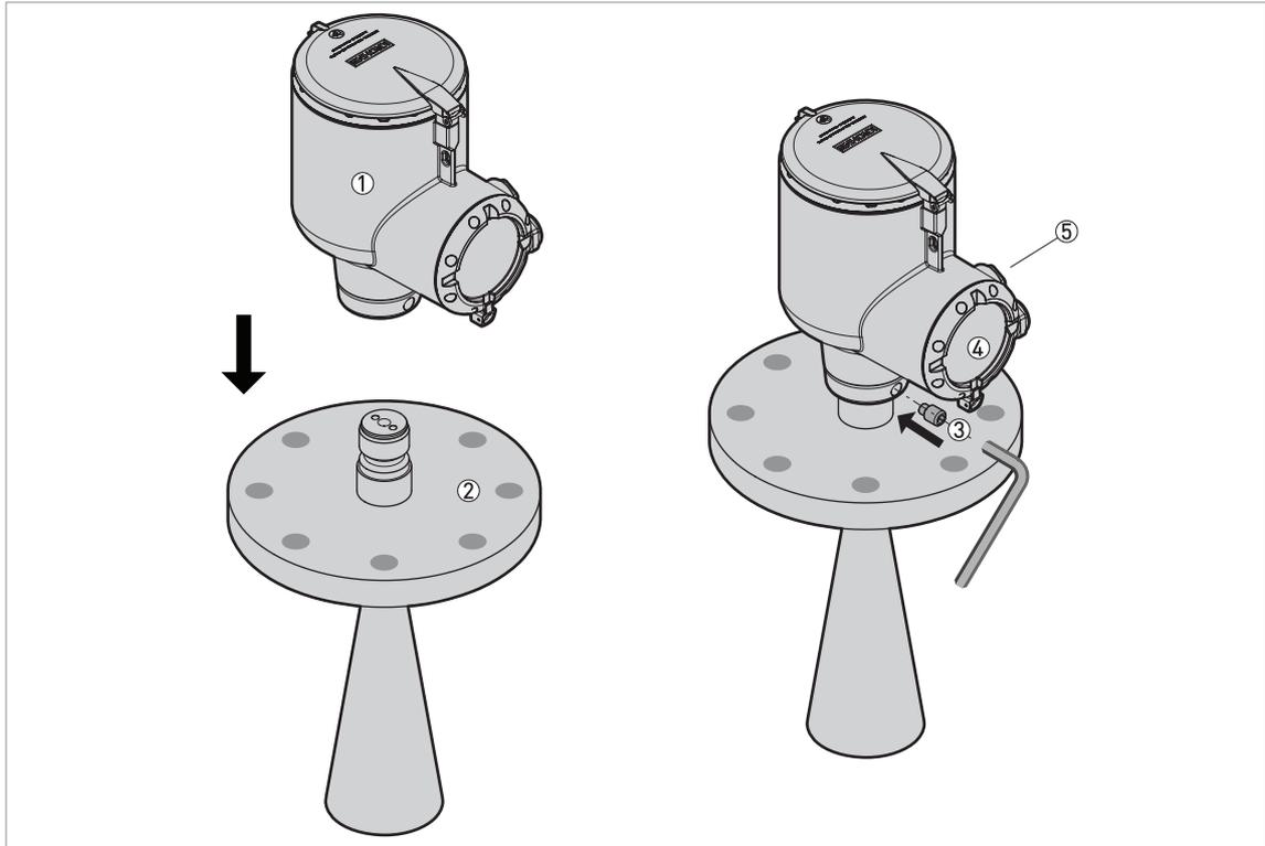
Figure 7-4: Procedure 3: How to attach the REFLEX RE Series signal converter
