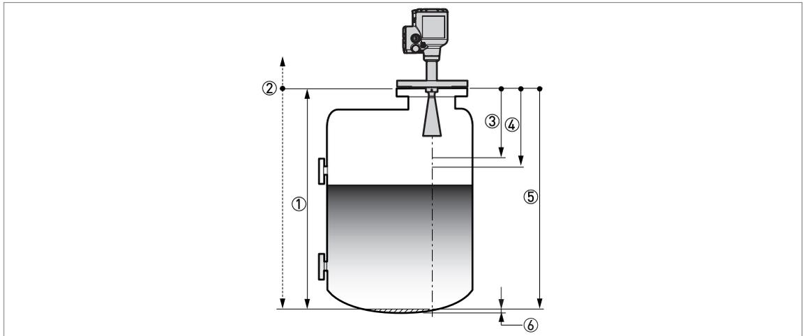
Figure 6-7: Distance measurement
