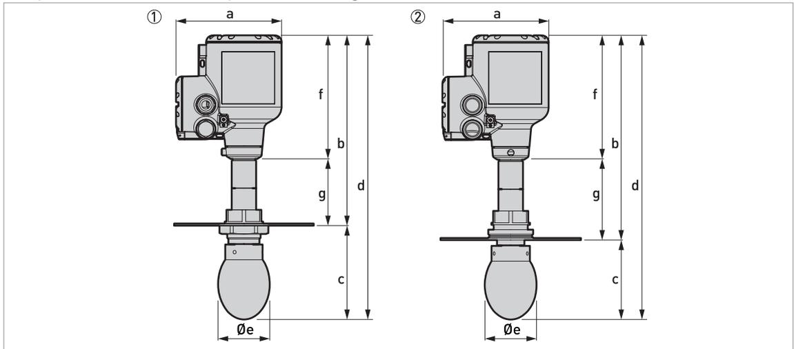
Figure 8-15: Drop antennas with low-pressure flange connections
