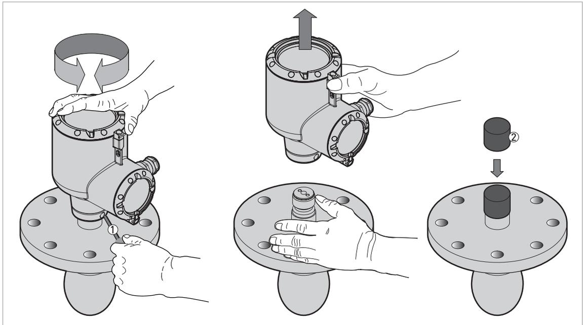
Figure 3-22: How to turn or remove the signal converter
