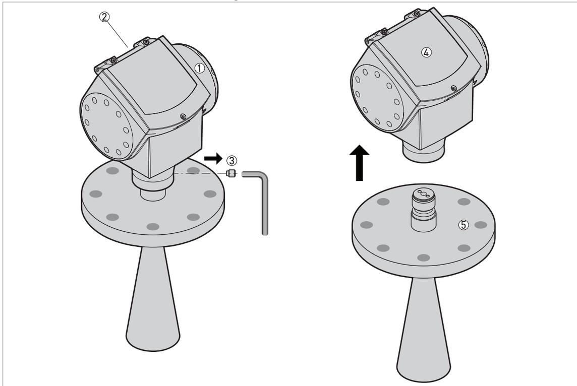
Figure 7-3: Procedure 2: How to remove the signal converter (VG7 radar level transmitter)
