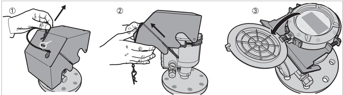
Figure 3-26: How to open the weather protection
