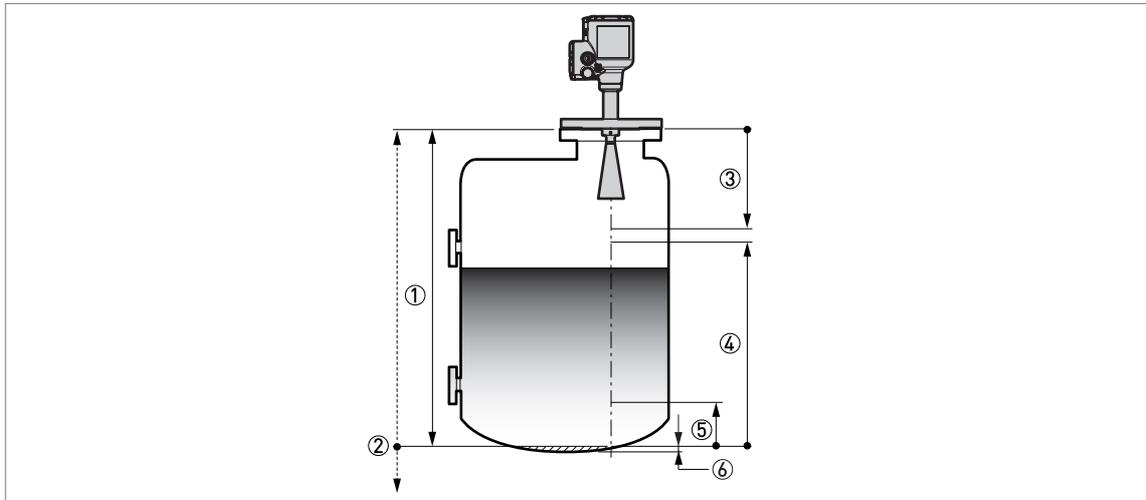
Figure 6-8: Level measurement
