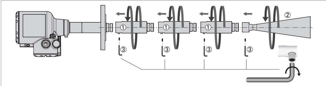
Figure 3-20: Metallic Horn antenna – how to attach antenna extensions
