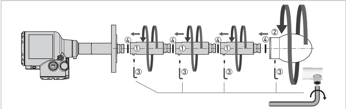
Figure 3-21: Drop antenna – how to attach antenna extensions
