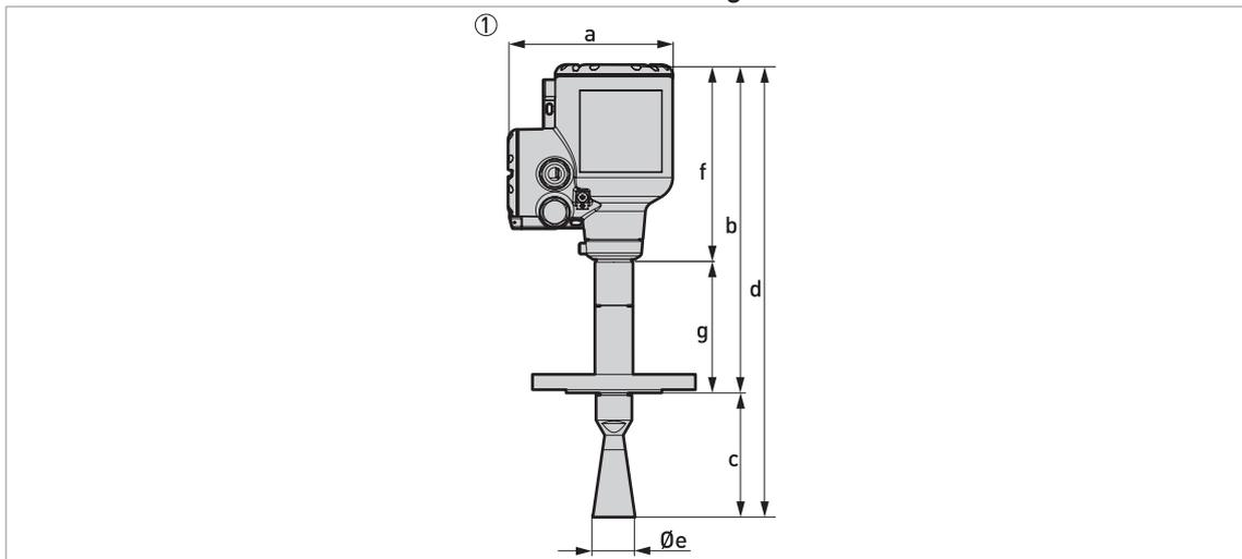
Figure 8-11: Metallic Horn antennas with standard flange connections
