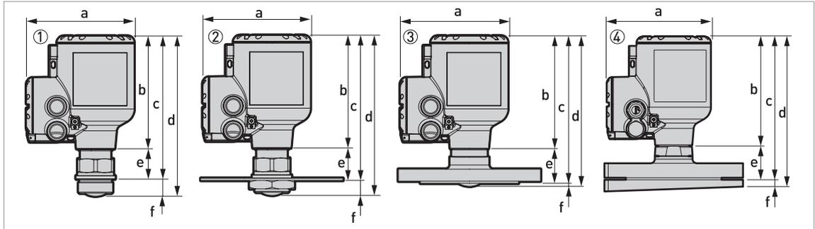
Figure 8-12: DN40 / 1½" Lens antenna versions
