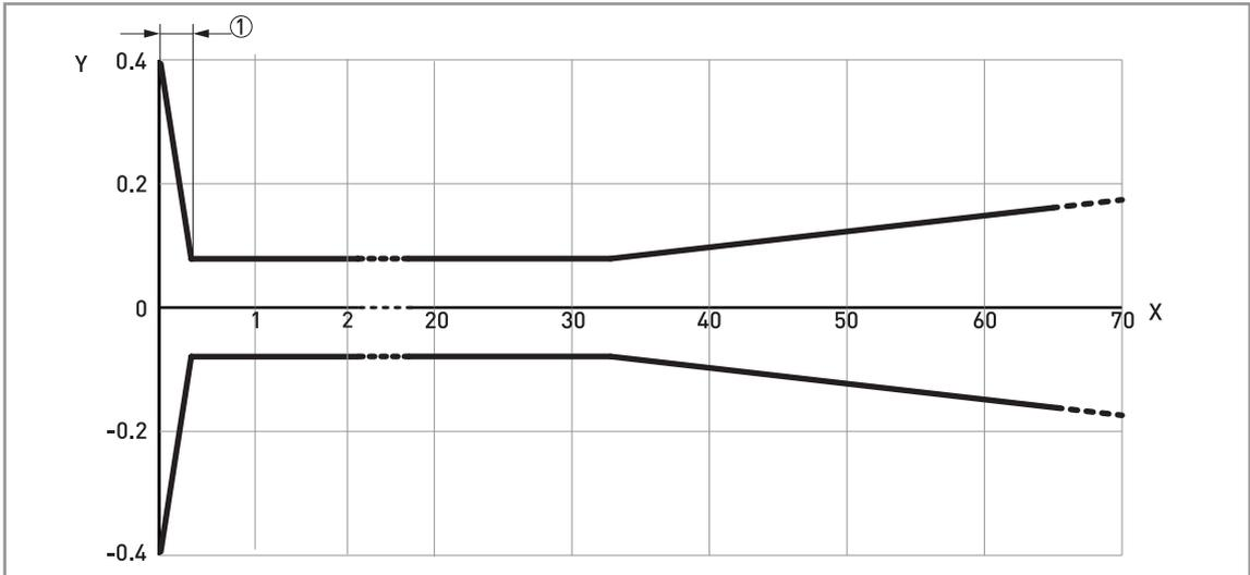
Figure 8-5: DN70 (1½") Lens antenna: measuring accuracy (graph of measuring accuracy in inches against measuring distance in ft)
