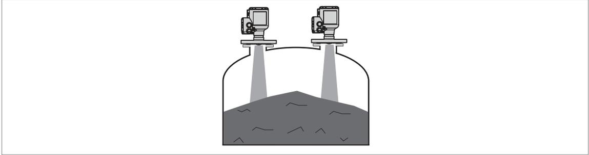
Figure 3-6: There is no maximum limit to the number of devices that can be operated in the same silo
