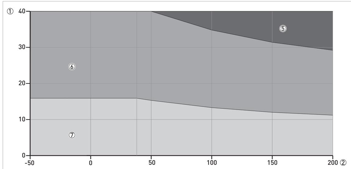
Figure 8-10: Pressure / temperature de-rating (ASME B16.5), flange and threaded connections, in °C and barg
