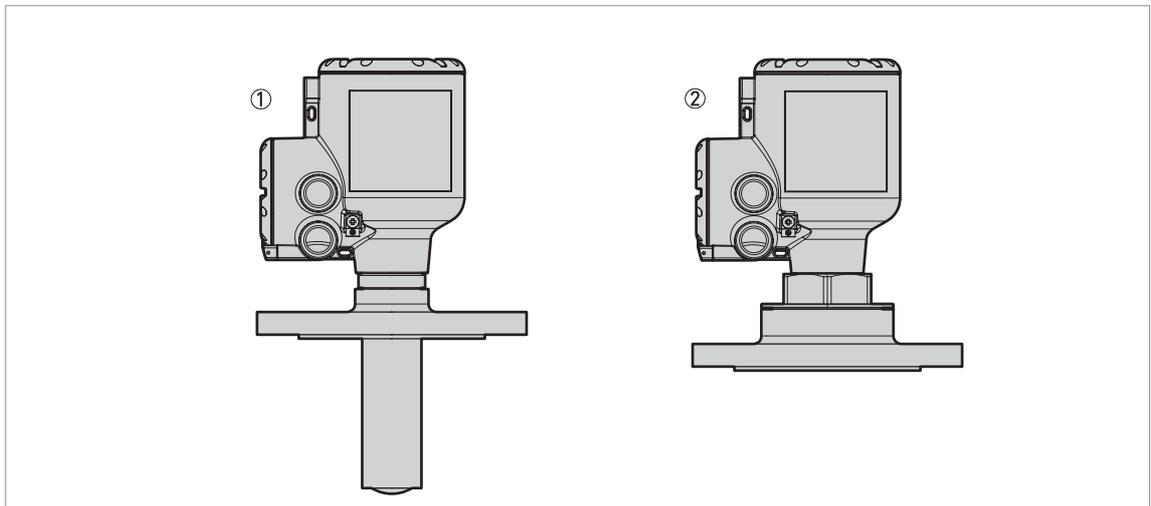
Figure 2-2: Types of antenna
