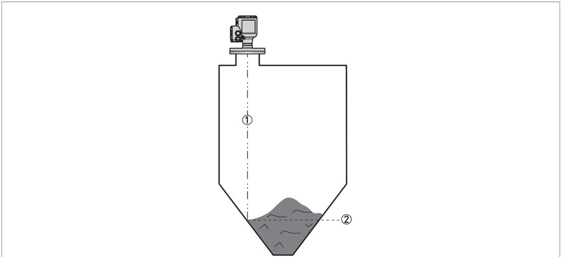
Figure 3-7: Tanks with dish-shaped or conical bottoms
