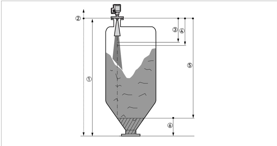
Figure 6-7: Distance measurement
