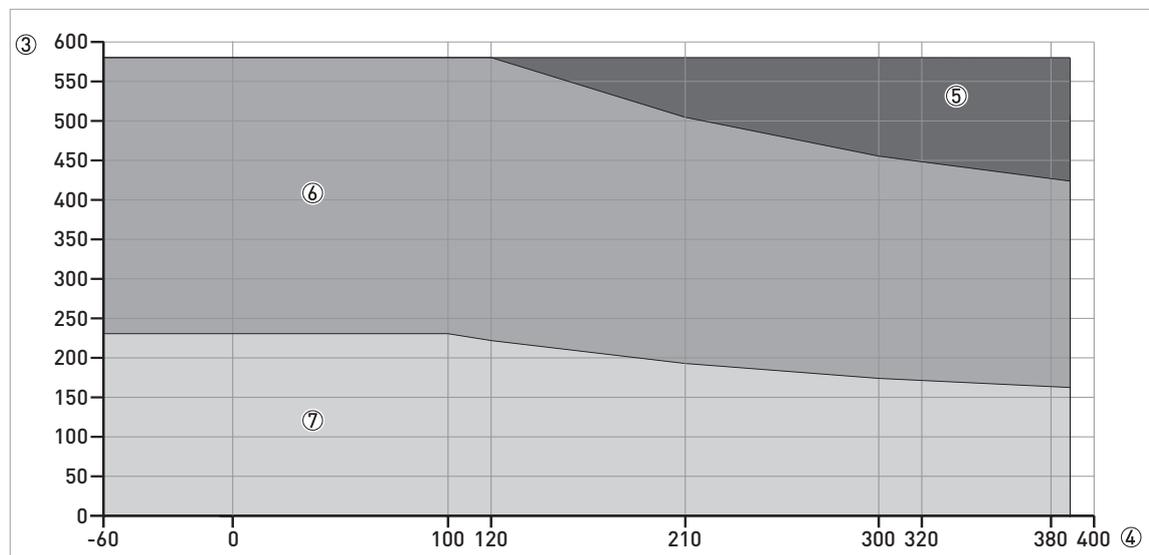
Figure 8-11: Pressure / temperature de-rating (ASME B16.5), flange and threaded connections, in °F and psig
