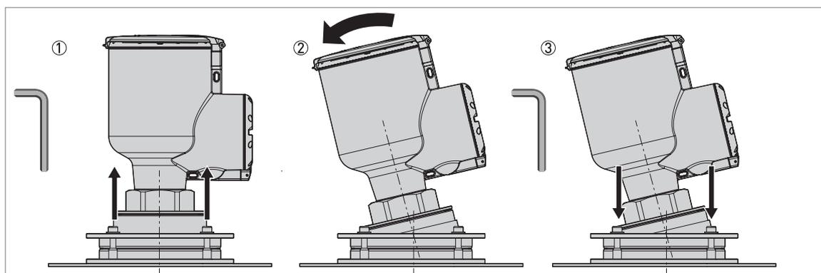
Figure 3-13: How to tilt the device
