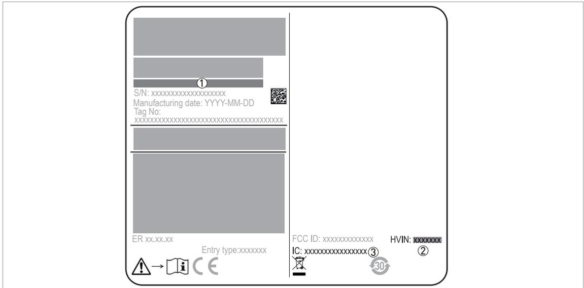
Figure 1-3: Canada: radio approval information on the nameplate
