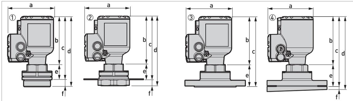
Figure 8-13: DN70 / 2<sup>3</sup>/<sub>4</sub>" Lens antenna versions
