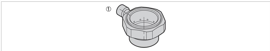
Figure 10-4: Accessories: purging system adaptor
