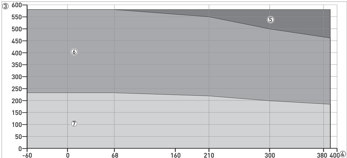
Figure 8-9: Pressure / temperature de-rating (EN 1092-1), flange and threaded connections, in °F and psig
