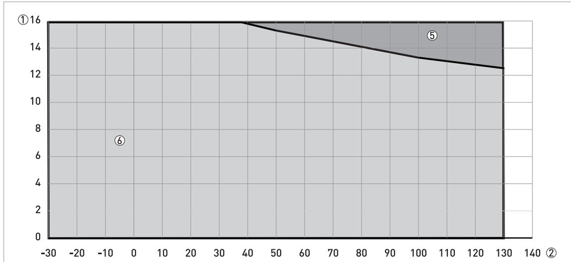
Figure 8-8: Pressure / temperature de-rating (ASME B16.5), flange and threaded connections, in °C and barg
