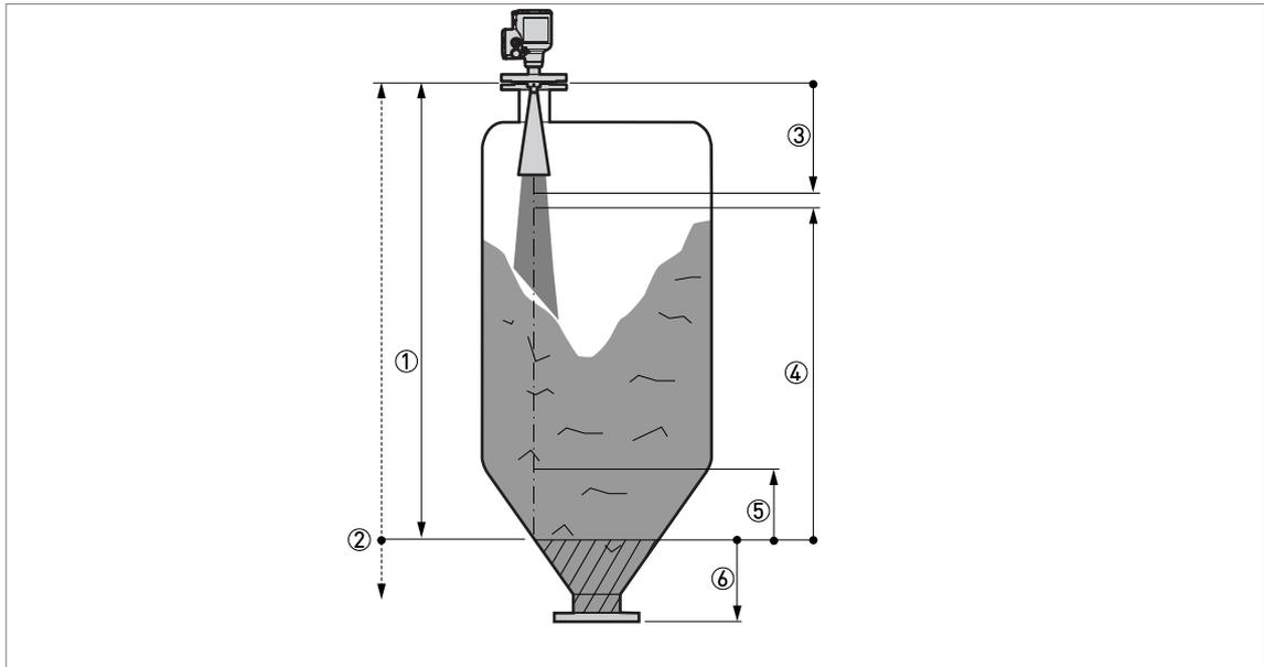
Figure 6-8: Level measurement
