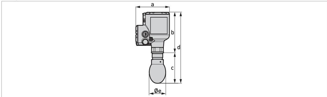
Figure 8-13: Drop antennas with threaded connections
