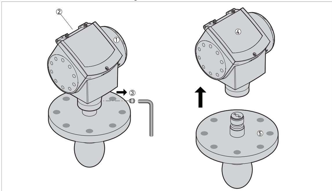
Figure 7-2: Procedure 2: How to remove the signal converter (VG6 radar level transmitter)
