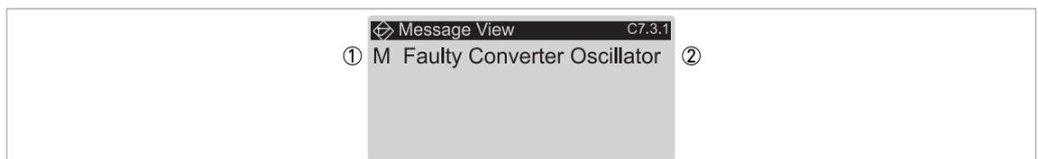
Figure 6-14: Description of the error (C7.3.1 Message View)
