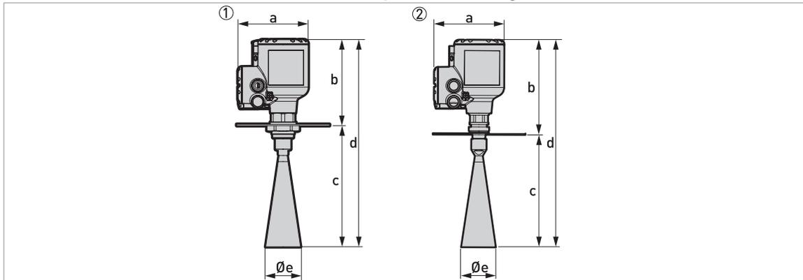
Figure 8-12: Metallic Horn antennas with low-pressure flange connections
