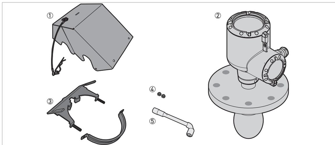
**Figure 3-20: Equipment needed to assemble the weather protection**
