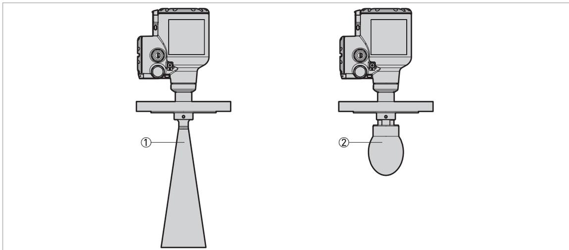
Figure 2-2: Types of antenna
