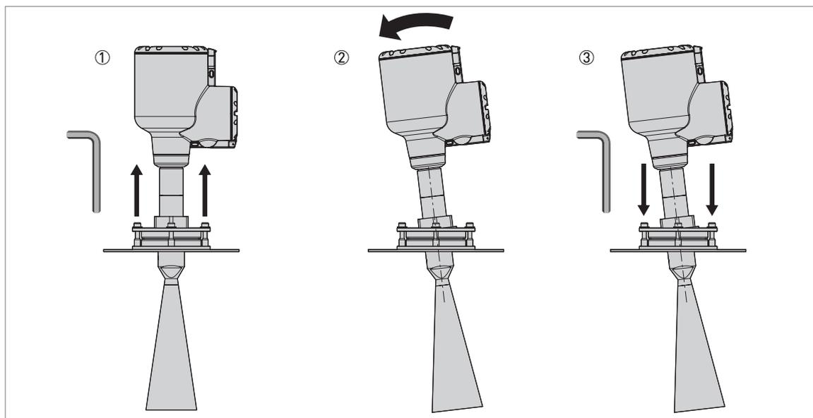
Figure 3-18: How to tilt the device
