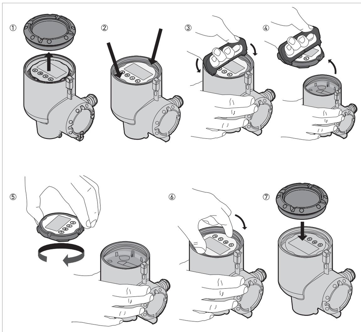
Figure 3-19: How to turn or remove the display module (option)
