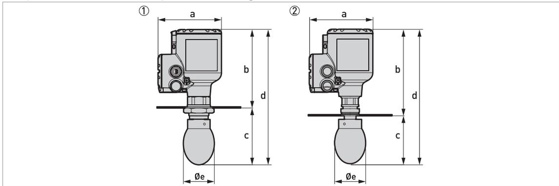
Figure 8-15: Drop antennas with low-pressure flange connections
