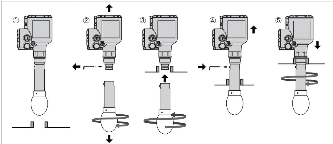
Figure 3-13: How to attach the device if the antenna is larger than the process connection
