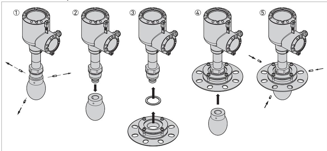
Figure 3-17: Device with a Drop antenna
