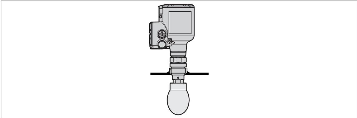
Figure 3-12: Threaded connections: installation procedure
