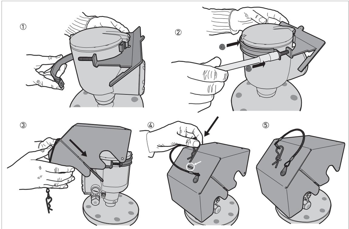
Figure 3-21: Installation of the weather protection
