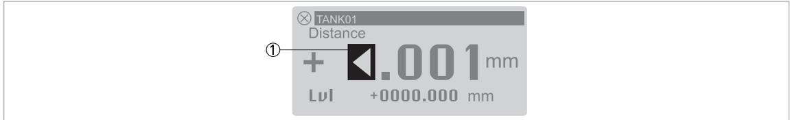
Figure 6-2: Error symbol: the number of digits and decimal places is not sufficient for the measurement data
