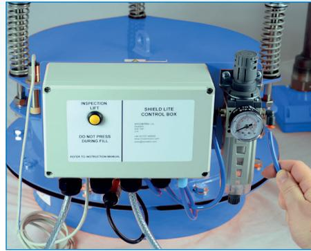
Figure 11: Connecting the air-line
